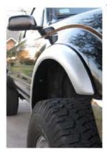
77-976 Fender flare edging is used to create a watertight seal between the fibreglass flare, bonnet scoop etc. and the metal guard on the body of the vehicle. The U-shape on the rubber goes over the fibreglass flare and the tail creates a seal against the body, as shown in the pictures
